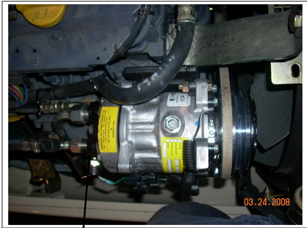
Horizontal “O” ring pad fitting and pressure switch attached to back of compressor.
