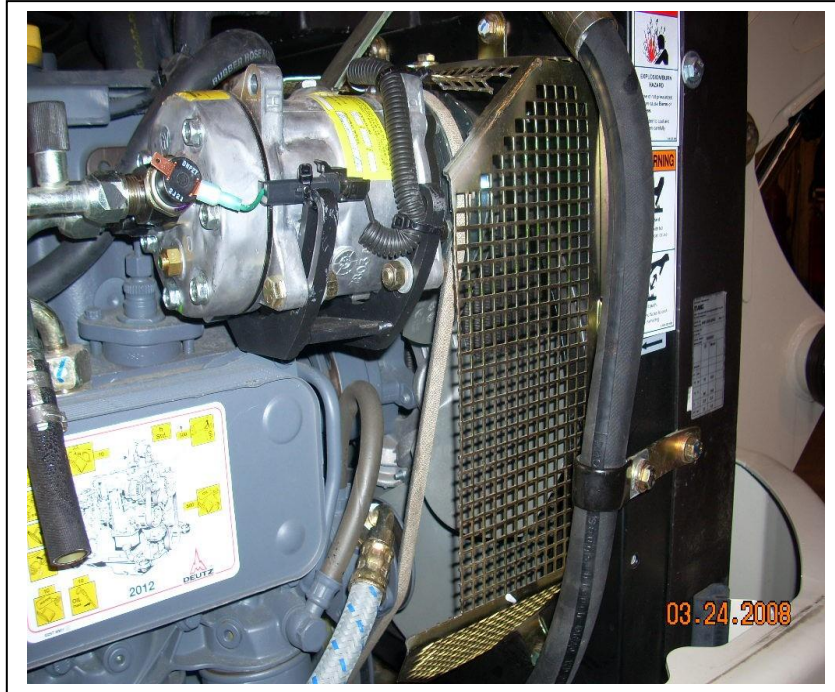
Compressor in place with guard in place. Modifications to the belt and fan guard are required to install the compressor.
