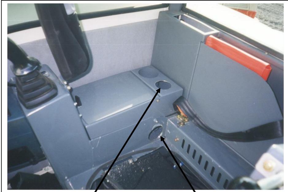
2 1/5" hole for snap-in louver
